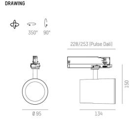
27 LED System perform. [W] Bulb type Luminous flux [lm] 2790 Current sec. [mA] 700 Colour temp. [K] 3000K CRI PREMIUM>90
