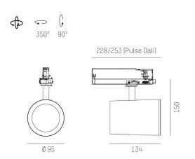
27 LED System perform. [W] Bulb type Luminous flux [lm] 2970 Current sec. [mA] 700 Colour temp. [K] 2700K CRI PREMIUM>90
